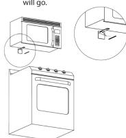
Drill 1/8" pilot holes in your pre-marked location on the wall. If you hit a wooden stud behind the drywall, use a #8 x 1.5" wood screw (not included) to complete installation.
