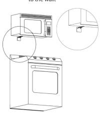
a. Find Auto-Out Microwave marked "L" for left. Insert adjustable bracket, with ridges of bracket facing up, into slat atop Auto-Out Microwave. Press down on pop-up tab to gently snap bracket into place.
