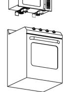
Measure to ensure a minimum of 9.5" from center of Left unit to center of Right unit. Confirm canisters are positioned over back burners.
