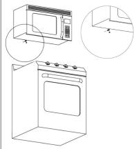
Align holes in wall-mount bracket with the installed anchors; insert the screws (provided) and use a screwdriver to tighten and secure wall-mount bracket to the wall.
