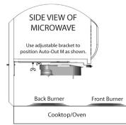
b. Lift Auto-Out Microwave unit to meet the wall-mount bracket, fastening the two wingnuts to join the parts together - tighten by hand to secure. Confirm canister is positioned over back burner. Repeat steps for right side of cooktop to complete installation.
