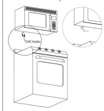
Screw in anchors into the pilot holes.
