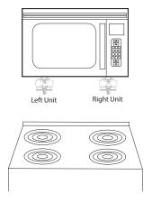
Measure to ensure you have a minimum of 9.5" from center of Left unit to center of Right unit.
