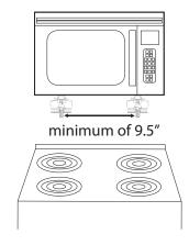
Installation is now complete. Ensure canisters are positioned over the back burners and the front of the unit extends over the front burner on each side.
