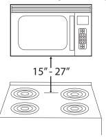
Measure from the cooktop surface to the bottom of the microwave to ensure required clearance of 15-27 inches. Insert bracket into slot atop Auto-Out Microwave for both units. Identify your Left & Right side units. Find the unit marked "R" for Right.
