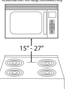
You will be attaching the wall-mount brackets to the drywall backsplash under the microwave. Center bracket over middle of left back burner. Use a pencil to mark through the holes where the screws will go.
