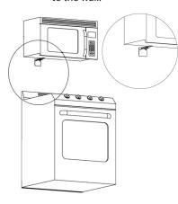
a. Find Auto-Out Microwave marked "L" for left. Insert adjustable bracket, with ridges of bracket facing up, into slat atop Auto-Out Microwave. Press down on pop-up tab to gently snap bracket into place.
