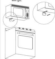
Drill 1/8" pilot holes in your pre-marked location on the wall. If you hit a wooden stud behind the drywall, use a #8 x 1.5" wood screw (not included) to complete installation.
