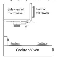
b. Lift Auto-Out Microwave unit to meet the wall-mount bracket in back. If applicable, connect magnets in front to the underside of microwave. Fasten the two wingnuts to join the parts together - tighten by hand to secure. Repeat steps for right side of cooktop to complete installation. Confirm canisters are positioned directly over the back burners.
