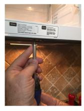
2.a Find the screws of the metal panel underneath the microwave (where the filters are located).
