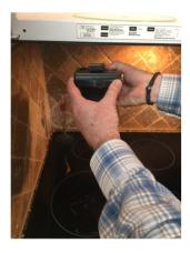
Open the microwave door; center the Left Auto-Out Microwave (marked L) over the middle of the front left burner and lift up.
